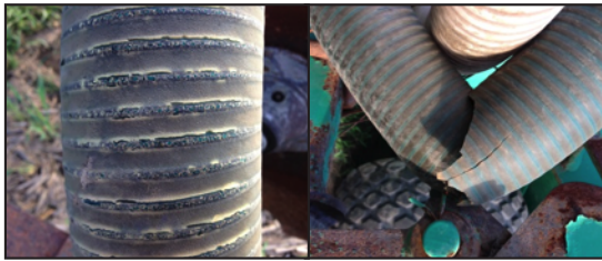
PVC Hose cracking due to UV exposure
